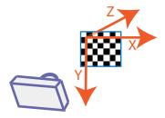
When you reconstruct a 3-D scene from multiple views containing a calibration pattern, the resulting 3-D points are defined in the pattern-based coordinate system. The "Structure From Motion From Two Views" example shows how to reconstruct a 3-D scene from a pair of 2-D images containing a checkerboard pattern.
